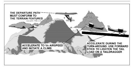
RULE OF THUMB: WHEN THE RUNWAY LENGTH IS DOUBTFUL, MARK THE MIDPOINT OF THE RUNWAY. IF 71% OF THE TAKEOFF SPEED IS OBTAINED AT THE 50% POINT ON THE RUNWAY, SUFFI-CIENT RUNWAY IS AVAILABLE FOR THE TAKEOFF. IF NOT, ABORT THE TAKEOFF AND WAIT FOR BETTER CONDITIONS. (COOLER TEMPERATURE, MORE HEADWIND, OR OFF-LOAD SOME PASSEN-GERS AND BAGGAGE, FERRYING THEM OUT IN SEVERAL TRIPS.
