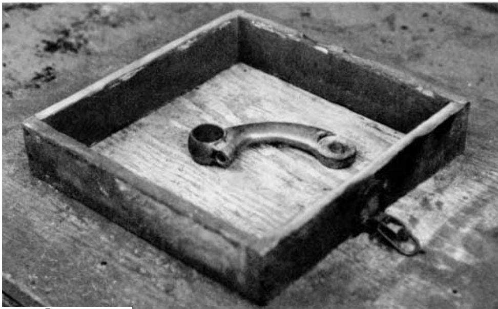
Fig. 6-9. The pattern, an original part, is laid on the molding board approximately centered in the drag. The holes in the part have been partially filled with clay to prevent unpredictable sand separation at these points during the molding process.
