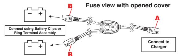
WARNING: ALL batteries MUST be CHARGED INDIVIDUALLY and properly tested to ensure they are in good condition (no dead-dying cells or excessive sulfation) before using this 210AY battery connector to maintain them in multiples. Only healthy, fully desulfated batteries should ever be MAINTAINED in sets of 2 or more.
