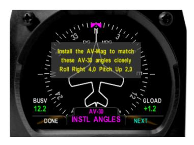
Adjust the AV-Mag mounting attitude to match that of the AV-30 as closely as possible. Simultaneously, the AV-Mag should be oriented as parallel to the line of flight as possible.
