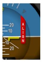
Figure 28 - Aligning Annunciator
