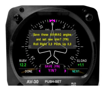
After roll and pitch angles have been entered, calibration may begin. Record the installation selections and parameters in Table 13-3 of Section 13.2.4.
