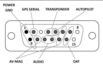
Figure 12 - Unit Connections – DB-15, Male (Rear Unit View)
