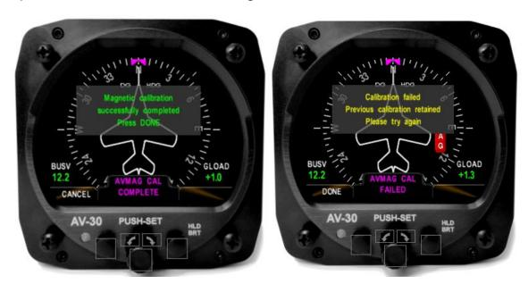
Figure 39 - AVMAG CAL Success and Failure Screens
