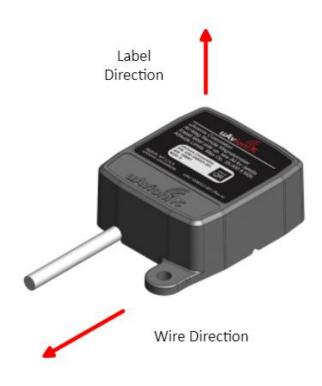
In addition to the installation orientation, the mounting attitude of the AV-Mag must be determined as well. Though a small amount of angular mismatch between the installation attitudes of the AV-Mag and AV-30 is tolerable, the AV-Mag is ideally installed with the same roll, pitch, and yaw as the AV-30.
