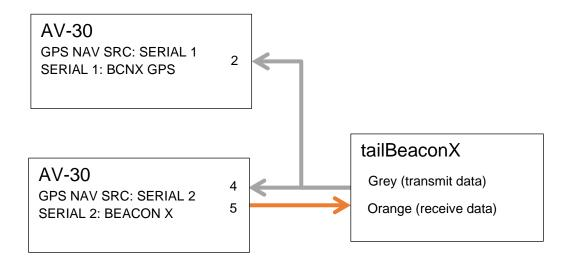
Figure 26 - Parallel tailBeaconX GPS Connections
