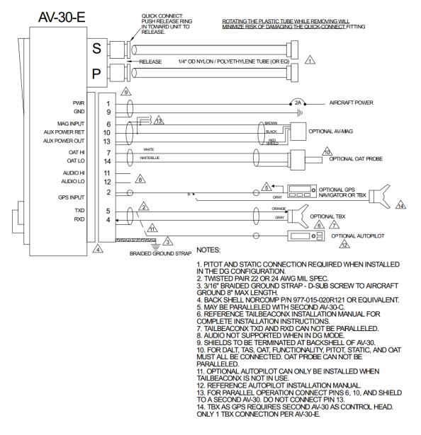
Figure 8 - Wiring Diagram - DG Position Installation
