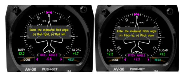
Once these values are committed, the AV-30 will calculate the differences in mounting angles for use in the heading solution. Once entered, changing these values without remeasurement of the AV-Mag angles will invalidate the installation calculation.
