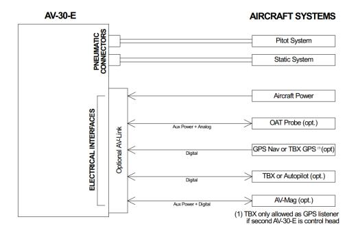
Figure 4 - AV-30 Aircraft Systems Interfaces - DG Mode
