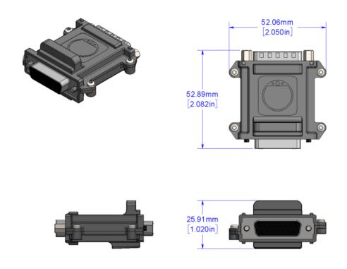
Figure 13 – AV-Link Mechanical Drawing
