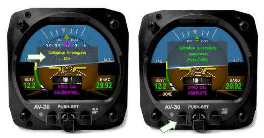
Figure 31 - Gyro Calibration Procedure
