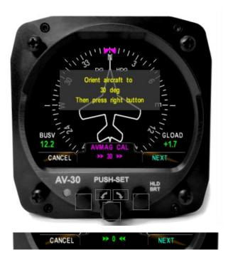
Figure 38 – AVMAG CAL Orientation Guide
