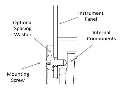
Figure 6 – Mounting Screw Dept Limits
