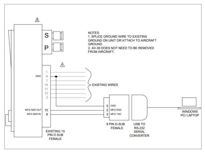
Figure 44 - Field Update Interface Diagram
