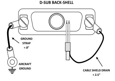
Figure 11 - Cable Shields and Ground Strap
