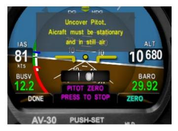
The PITOT ZERO function measures both the pitot and the static pressure sensor with identical air pressure conditions. Any difference in reading is saved and applied to subsequent airspeed calculations.
