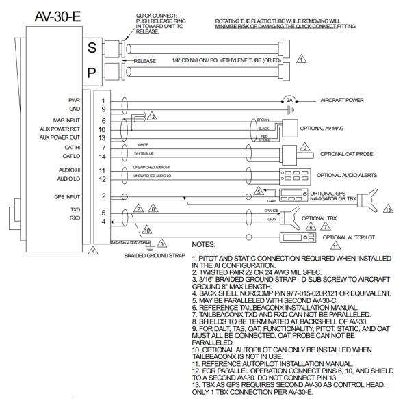
Figure 7 - Wiring Diagram - Attitude Indicator Position Installation
