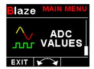
This menu displays the ADC value that have been read from the pressure sensor.
