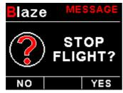
Press the F1/Up button during the normal display mode to manually start/stop a flight. This key is only active if the ASV-2 is setup to select the manual flight option under the "TIMERS" setup menu.
