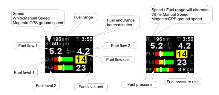
3.3 Single fuel flow and dual fuel level senders (dual tank) Single fuel flow, single fuel level sender, single calculated tank Differential fuel flow and dual fuel level senders (dual tank) Differential flow, single fuel level sender, single calculated tank Summed fuel flow and dual fuel level senders (dual tank) Summed fuel flow, single fuel level sender, single calculated tank
