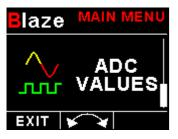
This menu displays the ADC values of the two fuel level and pressure sender.
