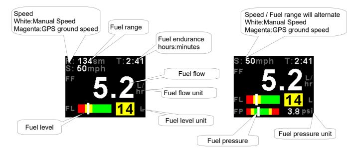
3.2 Dual fuel flow and calculated tank levels (dual tank) Dual fuel flow and dual fuel level senders (dual tank)
