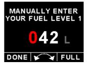
Press the F2 key during the main display screen to manually enter your current fuel level after fueling or defueling your aircraft. This function is only available if you have a mode selected where fuel level is calculated from fuel flow. Press the F2 key again as a "quick fill button" to the full level.
