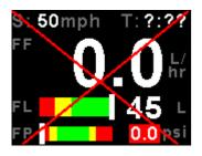
The red cross over the display means the FF-5 has lost communications with the external RDAC unit. Check the wiring between the FF-5 instrument and the RDAC unit. This error message is only available when the external RDAC is selected as the fuel data source.
