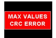
Max Values CRC error. Load default settings to restore to factory defaults. If the error message still persists then it could possibly be a non-volatile memory failure in which case the instrument will then have to be returned to the factory.
