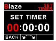
Press the F2 key to enter the set timer screen. Use the rotary control to set the countdown timer value. Press the F1 key to exit.
