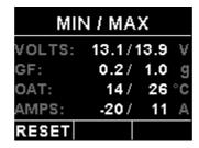
Press the F1 key to reset the maximum and minimum values. If the security option has been enabled, then the correct security code will have to be entered before you will be able to reset the maximum and minimum values.
