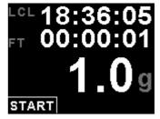
Press the F1 push button to start/stop the flight timer. This push button is only active if the flight timer is set to manual.
