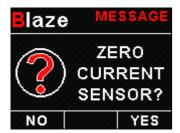
Select this function to indicate to the INFO-2 that zero current is flowing through the MGL current sensor. This is best done with the MGL current sensor disconnected from the main current supplying conductor.
