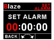
Press the F2 key to enter the alarm setting screen as shown on the left. Use the rotary control to set the alarm time. Press the F1 key to exit.
