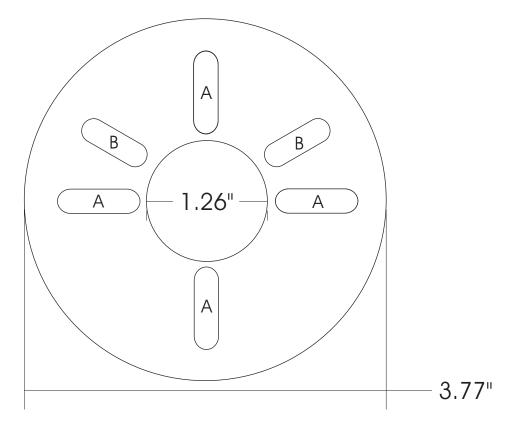
Slots A are used on 4-bolt patterns, slot dims of .860 x .245 Slots B are used on 3-bolt patterns, slot dims of .730 x .245
