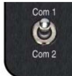
The up switch position is COM 1. Both pilot and copilot will be connected to the Com 1 transceiver. While in the COM 1 or COM 2 mode, the intercom functions normally. Both the pilot and copilot have transmit capabilities on the selected transceiver. All hear the selected audio if the intercom is in the ALL mode. Only the person who presses their Push To Talk (PTT), will be heard over the aircraft radio. Placing the toggle switch in the COM 2 position will place pilot and copilot on Com 2.
