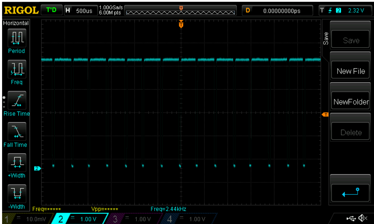
Tachometer Output of Fan at highest speed.
