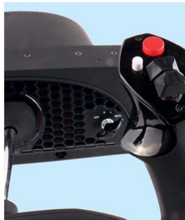
Above: A switch panel includes controls for external lights along with dual master and avionics master switches. Right: Twin rocker switches and two push buttons can be configured for a variety of functions. Left: Honeycomb's Alpha Flight Control yoke is arguably one of the most anticipated controllers to be released in recent years. Below: Control forces are fluid and smooth. An RJ-45 cable connects the base to the yoke as the wiring can't pass through the solid steel shaft.
