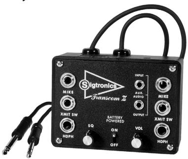
**FAIL SAFE RADIO COMMUNICATIONS:** Even with the intercom "OFF", the pilot can hear all radio communications and can transmit through the aircraft radio using the headset boom mic. The headset mic is routed directly to the radio via the "ON-OFF" switch. The "fail safe" feature also works should the battery go dead in mid-flight, thus providing the most fail-safe unit on the market.
